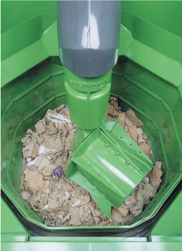
3. The special roller grips, tears up and compacts the material at a compression rate of up to 9 : 1 dependant upon waste streams.
