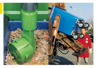
The Roto-Compactor grips, tears and compacts the waste by means of a specially designed steel drum. 2. The wheely bin is emptied by a dust car
